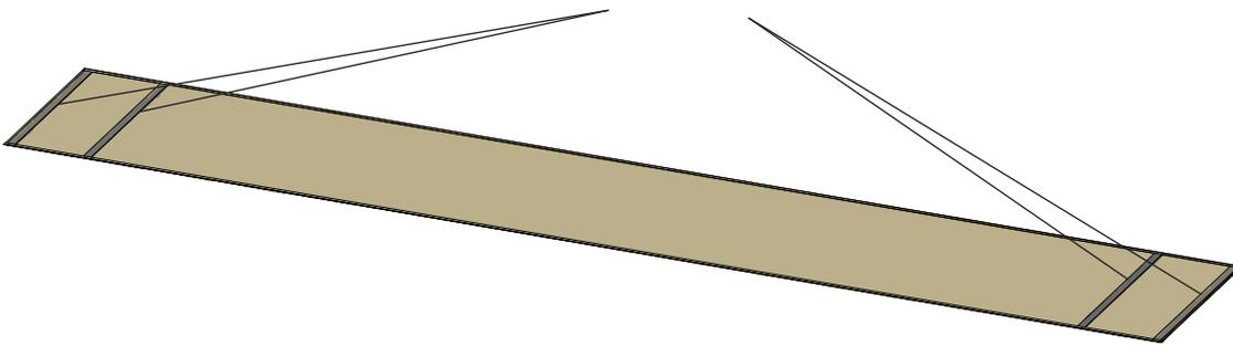
With the hook and loop fastener strips facing up, weave the canvas through the shade slats as shown. Note the pattern of the weave (below two shade slats, and above two shade slats). Starting with below one shade slat, and ending with the same.
