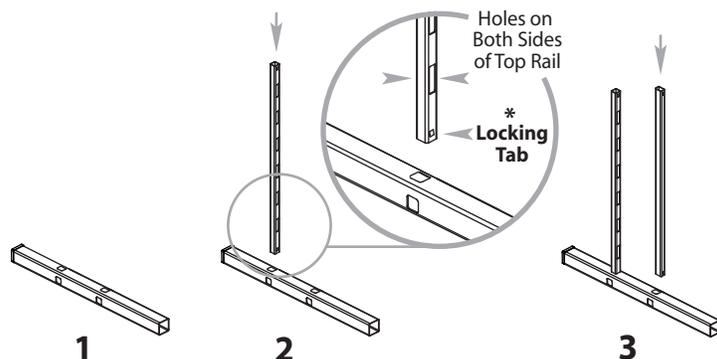
**\* Once rails are inserted into holes and pushed past locking tabs they will LOCK INTO PLACE PERMANENTLY.**
