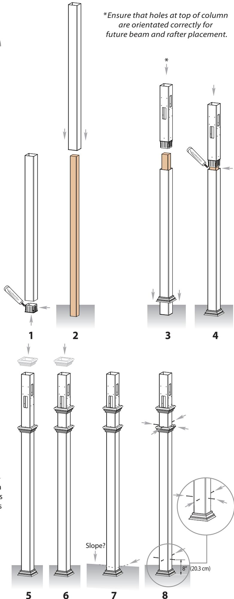
At this stage, the columns should be properly installed as per the following illustration, with the columns 88 1/2" in. (223.5 cm) apart.
