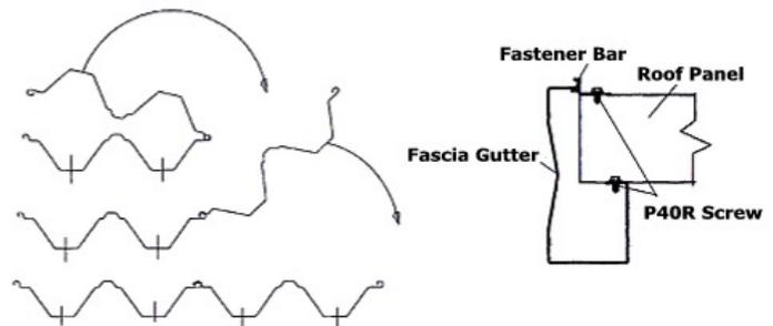
You may need to "squeeze" the pans slightly as you go in order to stay on the marks you have placed on the rear and front fascia gutters. The pans are designed to interlock by "rolling" the edge of each consecutive pan into the lock of previously installed pan.
