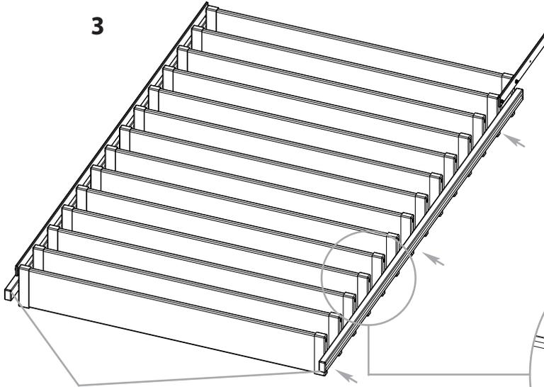
*The ends of the louver bars with large space should be at the same end.*
