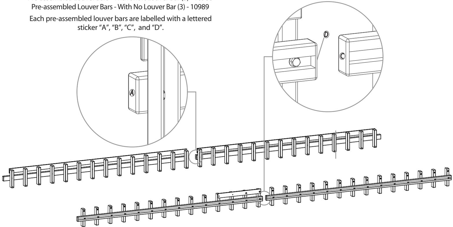
When assembling, match louver bar A with B, and C with D.
