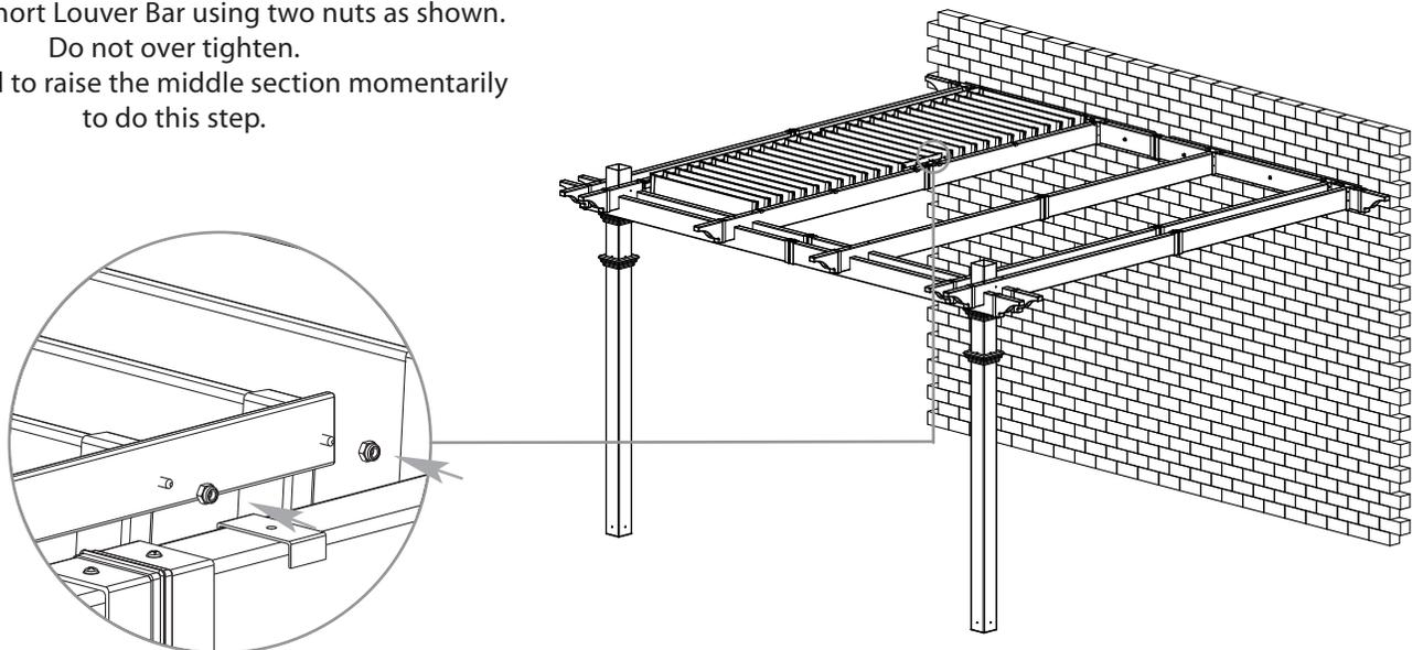
**Note: check that the holes are closer to the bottom as shown.**
