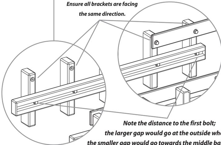
*Note the distance to the first bolt; the larger gap would go at the outside whereas the smaller gap would go towards the middle bar assembly.*
