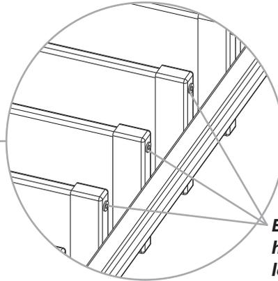
*Ensure that the holes in the louver holder brackets are all on top of the louver bars assembly*
